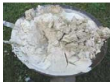
Addition of water = slaking
